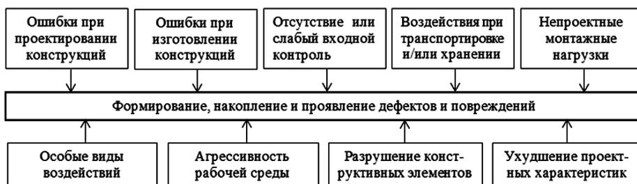
Fig. 1. Conditions for the manifestation of critical defects and damages
